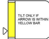
**WARNING** - Tilt Drum Only When Arrow is Within Yellow Bar. The indicator panel shown in Figure 2.2 is located on the safety screen above the push handle. When the arrow is within the yellow bar, the bottom of the upright drum will be between 6" and 12" above the floor. The operator should make sure the drum holder and drum will not come in contact with the floor, rack or other obstruction during tilting of the drum or the drum could be dislodged, dropped or the MORStak could tip over.
