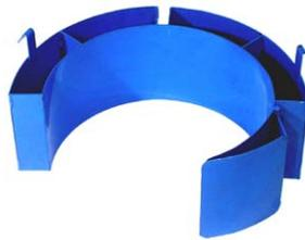
Diameter Adaptors for drums from 18.5" to 22" (47 to 55.9 cm) in diameter do not have hold-down brackets. They fit between the ribs of a steel drum. For plastic or fiber drum, use Diameter Adaptor in combination with the Bracket Assembly to prevent the drum from slipping lengthways through the drum holder.
